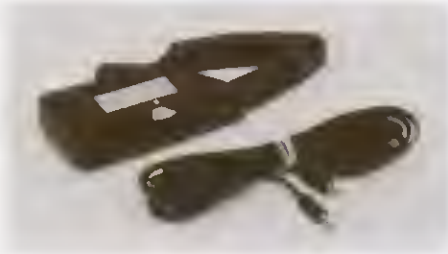
Model 1685 Clamp-On AC Probe (DMMs) Range: 2, 20 and 200A rms. Accuracy: \pm 4\% of range at 60Hz; \pm 6\% of range at 50Hz. Temperature Coefficient: \pm 0.05\%/^{\circ}\text{C} on 20A and 200A ranges; \pm 0.3\%/^{\circ}\text{C} on 2A range. Maximum Allowable Current: 300A rms. Maximum Conductor Voltage: 600V rms. Conversion Ratio: 0.1V/A rms.
