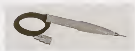
Model 6101A Shielded Test Lead: Straight through probe and shielded lead with 0.8m (30") of shielded low noise cable terminated by Teflon-insulated UHF connector. Use with 6012 adapter for Models 602, 614, 616 and 619.
