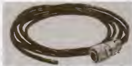
Model 1482 Low Thermal Input Cable: Similar to Model 1481; 3m (10 ft.) of cable terminated with a mating connector and bare copper leads, allowing the user to make his own special low thermal input connectors to Models 148 and 181.
