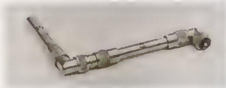
Model 2503 Static Detector Probe: Designed to detect voltage due to charge on relatively small surface areas. Solid coaxial 13mm (1/2 in.) diameter tube used with 89mm (3 1/2 in.) head, 89mm (3 1/2 in.) coupler, 25mm (1 in.) adapter and two 90° angle adapters which may be placed at various junctions along the tube. It gives a 10,000:1 ±10% division ratio when used with Model 610C and held 6mm (1/4 in.) away from a charged plane of at least 13mm (1/2 in.) diameter. Output is a UHF male plug.
