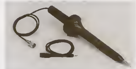
Model 6103C Voltage Divider Probe: Permits voltage measurement to 30kV and has a 1000:1 division ratio. Accuracy is ±5% of reading. Its 4.5 \times 10^{14} \Omega input resistance permits use with Keithley electrometers and other high impedance multimeters. Connector is a UHF male plug. Requires the 6012 Coaxial to Triaxial Adapter when used with Models 602, 614, 616 and 619. Lead length is 0.8m (30 in.).
