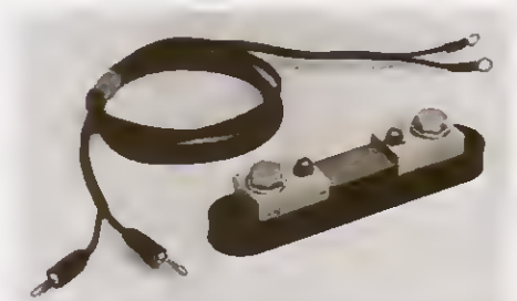
Model 1651 50 Ampere Shunt: External 0.001 \Omega \pm 1\% , 4 terminal shunt, extends current measuring capability of Keithley DMMs to 50A.
